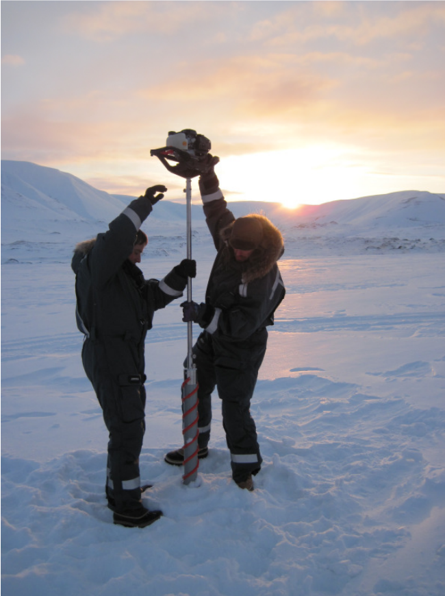
Drilling core for SWE measurements (Marco Möller, Roman Finkelburg)
