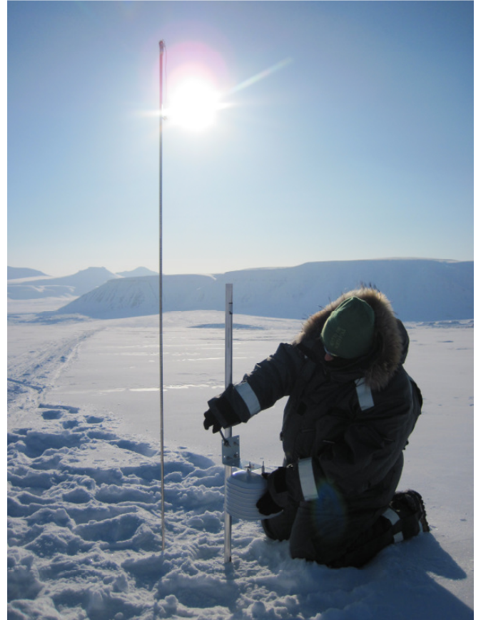
Mounting air-temperature sensor on ablation stake (Rebecca Möller)
